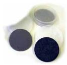
Always use protection filters to protect the measuring sensor from undesired particles or aggressive substances. If your samples could emit volatiles it is necessary to use chemical protection fitlers. The filters can be fit with the tension ring and provide protection against different substances in gaseous form.
