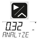
The measurement is started by pressing the "Start/Stop" button. Once pressed, the analysis function is initiated and the display shows "ANALIZING". As long as it is flashing alternately (Analizing/ ...°C) the aw-value and the temperature are not stable. The result can be read at earliest when the "stable"-value is displayed. An acoustic signal indicates the end of the measurement.
