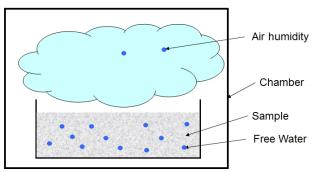
This exchange process ends in equilibrium where the mass transfer of free water to the air is equal to air humidity diffusing back to sample. At this point the measurement can be taken. If taken earlier, it might be that more free water is in the sample than in the air and this results in a wrong value.
