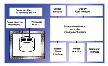
The *LabStart-aw* consists of modular assemblies in combination with the unique resistive electrolytic Novasina measurement technology, which is built inside the aW sensor. The aW measurement signal is electronically processed together with the NTC-based temperature measurement. Afterwards it is further processed by a high capacity micro controller. This is handling the LCD display unit. The mains are supplying the whole electronics with power.
