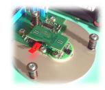
The **LabStart-aw** contains sensitive electronic assemblies. Please protect these items from electrostatic discharge (esd) by discharging yourself at a grounded, conductive surface (e.g. radiator) before you open the housing of the instrument.
