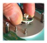
**Important:** Make sure you mount back the cover correctly. Special care has to be taken for the 4 screws fixing the cover to the cover plate. Screw them tightly. If cover is not closed properly, measurement problems can occur
