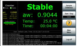
Once the measurement is stable, it will be displayed in green colour and indicated by a green LED. All the information as aw-value, temperature and stable time are displayed.
