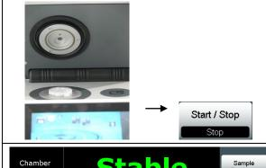
Place product sample in the measurement chamber, close cover and press the start button in the main menu screen. The instrument switches then to the measurement screen. A yellow-coloured LED is blinking indicating that the measurement is currently ongoing as well as "Analyzing" is displayed in the start/stop button.
