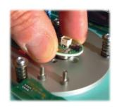
**NOTE:** The upper measurement chamber plate is still connected to the lower housing by a ribbon cable. Do not loosen or remove the ribbon!
